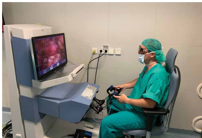
Figure 2. The position of surgeon at the operating console. Camera is controlled with the eye tracking technology, while the other two robotic hands are controlled with the laparoscopy-mimicking instrument handles. The console is equipped with haptic feedback and ultra-high-definition 3D screen.
