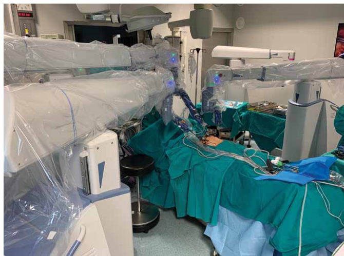
Figure 1. Robotic setting in the operating theatre. There are three robotic hands controlled by the operator. One is holding the camera and the other two are holding instruments. Additional trocars are used for laparoscopic instruments controlled by assistant surgeons.
